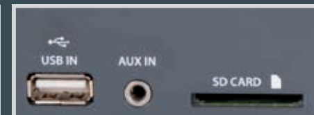
Additional external connections: USB port, aux. input and SD card slot.
