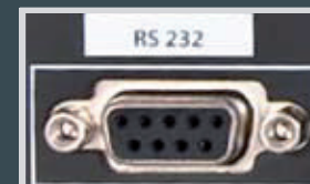
RS 232 connexion for external control of the different functions.
